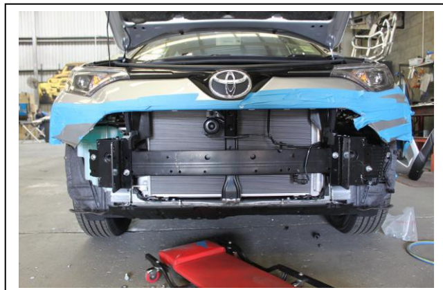
Figure 2: Disconnect bottle from passengers side inner guard
