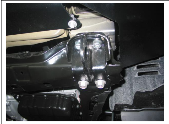
Figure 17: Tow hook installed onto under body frame
