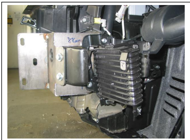
Figure 5: Oil cooler mounted to passengers side outer.
