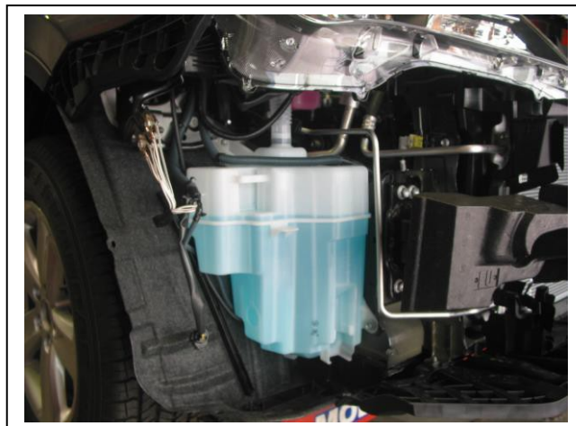
Figure 2: Disconnect bottle from passengers side inner guard
